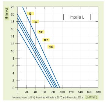
Please remember that the delivery rate is reduced as the **viscosity** increases. The **density** of the pumped liquid similarly affects the delivery rate, though to a lesser extent.
